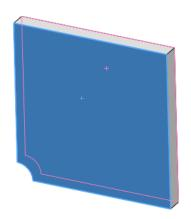
9 Using the identical procedure apply a symmetry fixture to the other edge shown in the figure. This time use Plane2 feature for Face, Edge, Plane, Axis for Direction field.
