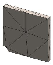
This large value for the global element size is used to demonstrate how the h-adaptive method refines the mesh to get accurate results.
