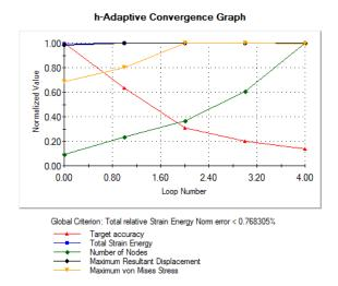
**Note:** To further improve the accuracy of the solution, it is possible to continue with the h-adaptivity iterations by initiating subsequent study runs. Each subsequent study run uses the final mesh from the last iteration of the previous run as the initial mesh for the new run. To try this **Run** the H-adaptive study again.
