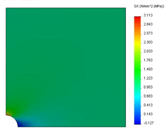
The analytical value for the maximum normal stress is  $\sigma_{max}$ = 3.113 MPa (451.5) psi.
