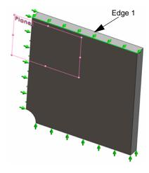
After applying all fixtures, two items: (Symmetry-1) and (Reference Geometry-1) appear in the Fixtures folder.
