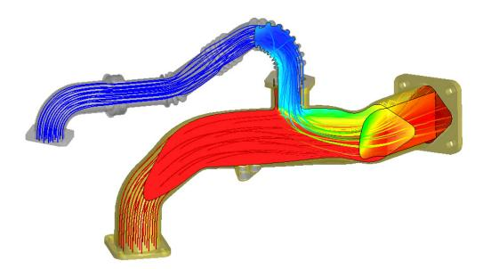
Fluid Mixing Analysis in CAD Embedded CFD Simulation solution
