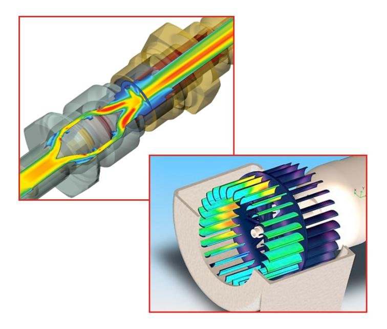
For several decades engineers and mathematicians have been trying to improve the understanding and prediction of fluid dynamics and heat transfer phenomena by means of Computational Fluid Dynamics (CFD) simulation. The objective is clear - to optimize the design of products and processes that involve fluid flow while minimizing the experimental effort, time and cost expended.
