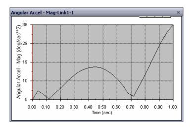
The results indicate the maximum angular velocity and angular acceleration of 6 deg/sec and 38 deg/sec^2, respectively.
