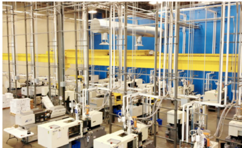
The lights-out injection molding machines that continually work to allow Eldon James to compete with offshore competitors.
