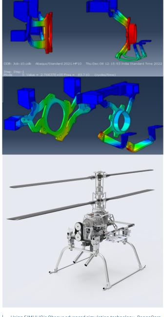
Using SIMULIA's Abaqus advanced simulation technology, RangeAero engineers can simulate the effects of all of the different types of physical phenomena that affect rotorcraft performance, including nonlinear structural analysis, rotor dynamic analysis, dynamic drop simulations on landing gear, nonlinear contact analysis, and nonlinear materials (Such as composites, carbon fiber, metal alloys.) analysis, including plasticity, viscoelasticity, and fatigue analysis.
