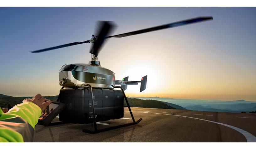
RangeAero engineers relied on SIMULIA's Abaqus advanced simulation technology to develop their Jestar autonomous freight helicopter, for regional commercial and military transport applications. They used the powerful analysis capabilities to ensure the design withstands the loads and stresses induced by aerodynamic forces without resorting to lengthy, costly prototyping iterations, which helped the company shorten time to market.
