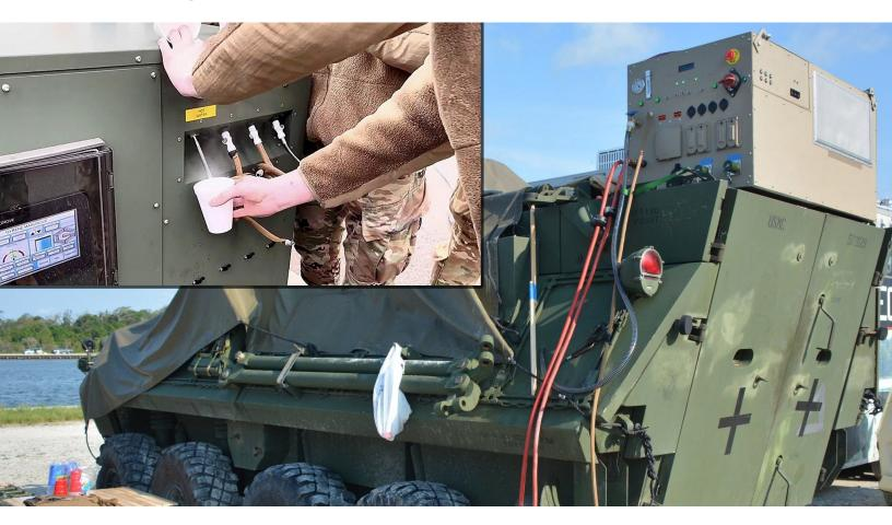
Gyrene leveraged **3D**EXPERIENCE Works design, data management, simulation, collaboration, and communication solutions to develop its innovative Mangrove Vehicle Integrated Atmospheric Water Harvester for the U.S. Marine Corps. The system creates water from the atmosphere in even the most arid climates, and also includes a mobile filtration system that produces purified drinking water from any water source, whether salt, brackish, or contaminated by pollutants.
