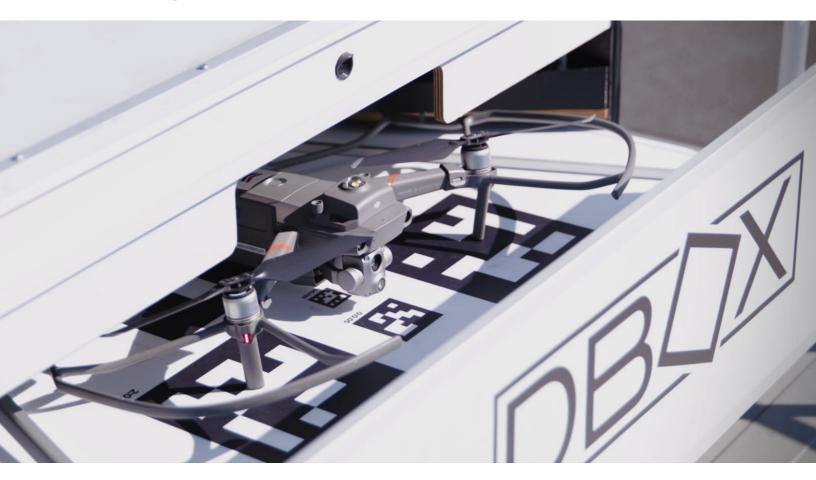
DBOX relied on SOLIDWORKS and **3D**EXPERIENCE Works product development solutions to develop its innovative Drone-in-a-Box invention, which is installed on rooftops across Europe to house, control, and automatically change drone batteries via a robotic arm, protecting drones from weather and enabling drone operations with little or no human interaction. The **3D**EXPERIENCE platform supported DBOX during its fast, collaborative development process.
