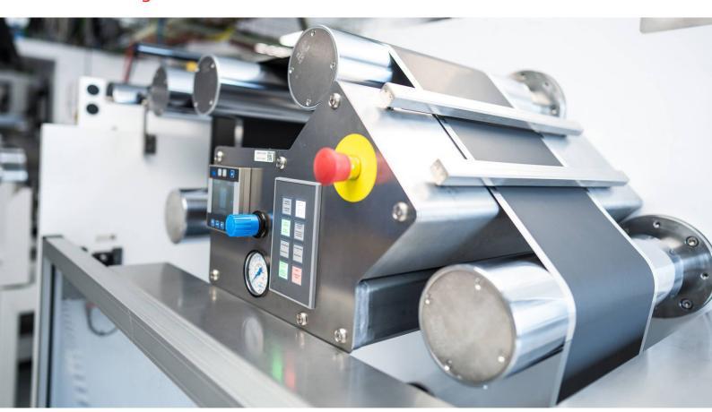
Using **3D**EXPERIENCE SOLIDWORKS and expanded portfolio solutions, AM Batteries is innovating a dry coating method for making Li-ion battery electrodes that is safer, less costly, and less environmentally harmful than the dry coating solvent-based slurry-coating methods that are currently used to make Li-ion battery electrodes, including those that are used on EVs.
