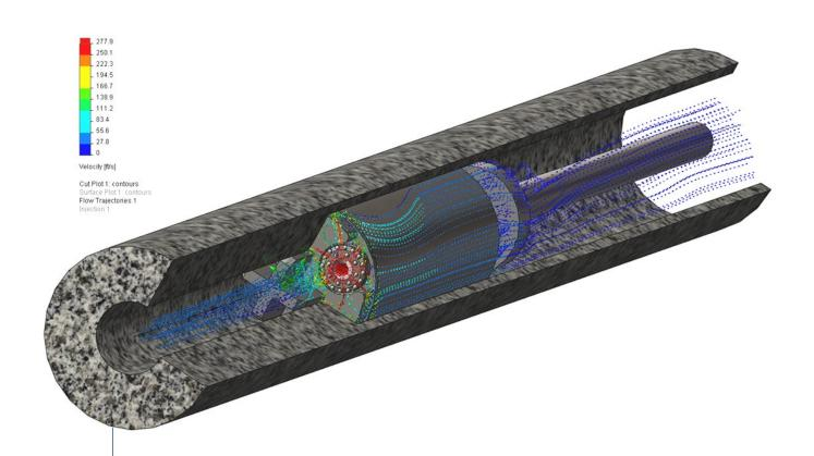
With the results of a SOLIDWORKS Flow Simulation study, Center Rock customized its percussive rock bit design to let cuttings fall by gravity, accelerating the rescue of 33 trapped Chilean miners.
