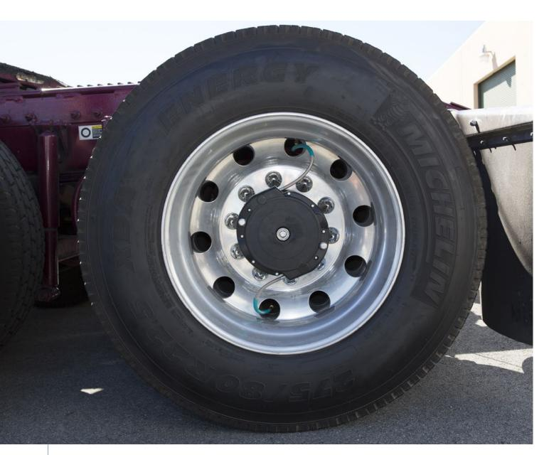
Using SOLIDWORKS design, analysis, CFD analysis, plastics injection-molding analysis, and technical communication solutions, Aperia Technologies has developed a revolutionary automatic tire inflation technology that utilizes a wheel's rotational motion to maintain optimal tire pressure.
