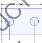
Dimensioning from the edge and from center to center will maintain the distance between the hole centers and allow it to be changed that way.
