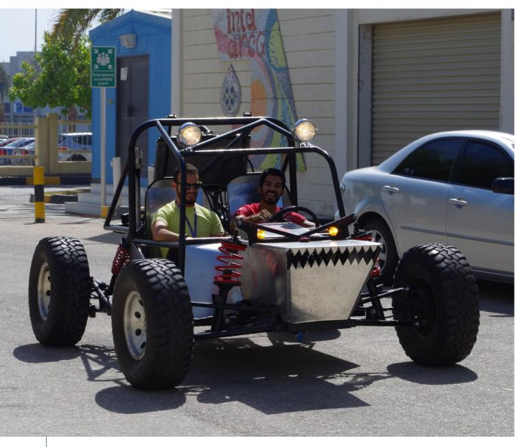
Above is Bahrain Polytechnic's first completed car—a desert buggy. It was designed from first principles, analyzed, developed, and manufactured by mechanical engineering degree students using SOLIDWORKS software.
