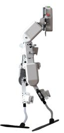
Using SOLIDWORKS development tools, Angel Robotics has grown rapidly, quickly launching two products: the WalkON Suit for completely paralyzed individuals, and ANGELEGS, a lower-extremity assist robot for people with partial walking impairment.
