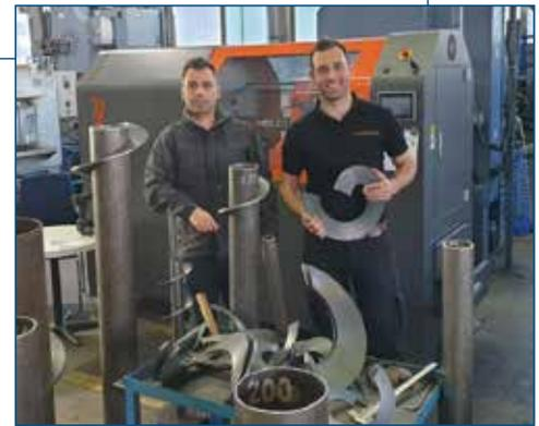
With SOLIDWORKS simulation capabilities, RoboHelix engineers were able to dial in the force required, and in what direction it should be applied, to achieve the controlled deformation through which the company’s robotic flight-forming machine stretches a metal disc to form a helical flight.
