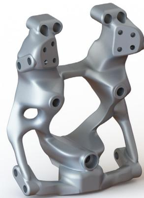
With SOLIDWORKS Simulation Professional topology study capabilities, Giaffone Racing is designing new components for the Brazilian Stock Car series, beginning with the suspension upright, or knuckle, shown here, which attaches the wheel, brake rotor, hub, brake caliper, and steering arm to the vehicle. With a SOLIDWORKS topology study, Giaffone optimized this component to reduce weight while maintaining stiffness.
