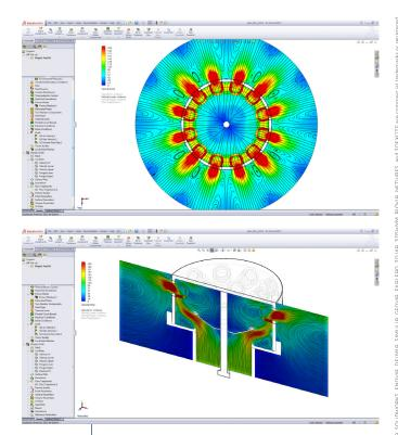
Using SOLIDWORKS Simulation Professional and SOLIDWORKS Flow Simulation software, Penn-Troy Manufacturing simulated the structural, vibration, and explosive gas effects of a crankcase explosion to improve the performance of its Bicera relief valves, cutting weight and improving performance while simultaneously reducing prototyping costs.
