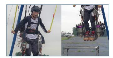
Using SOLIDWORKS Topology Optimization studies to reduce weight in several components and SOLIDWORKS Flow Simulation tools to optimize the shape of the patented thrust vector nozzle for the four jet engines—two for each leg—Exovolar was able to complete its first hovering test without undue rounds of prototyping by simulating design performance and optimizing the design in software.
