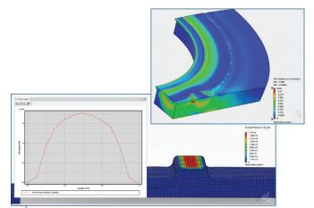
Using **3D**EXPERIENCE SIMULIA SME solutions, Morgan Polymer Seals has realized faster simulation turnaround times and reduced simulation costs, despite conducting a substantially larger volume of complex simulation studies, such as contact and hyperelasticity
