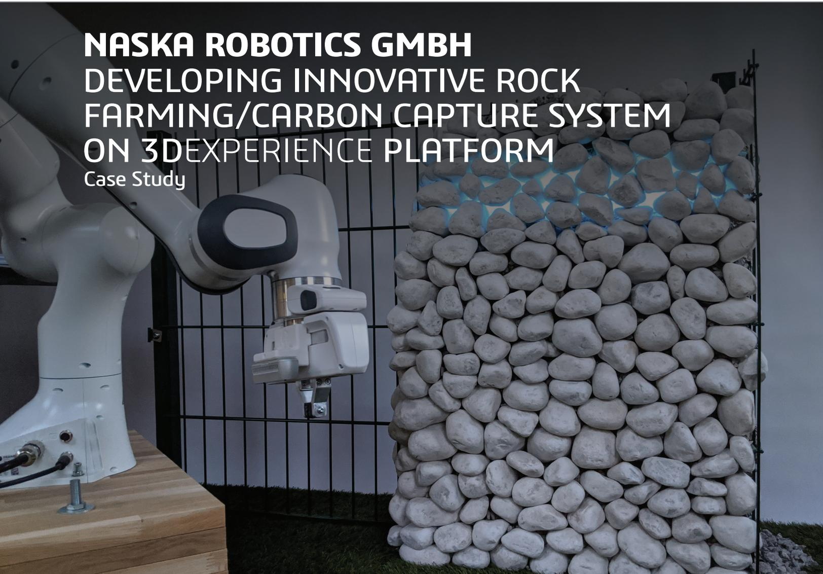
NASKA robotics is leveraging the cloud-based **3DEXPERIENCE** platform to complete research and development of its RockFarm robotic system for the mineralization of carbon dioxide to fight the effects of climate change. The robotic system will build rock walls, fill them with rock particles of less than 20 microns in size that absorb carbon dioxide, flush the walls once the rock medium becomes saturated with carbon, and then refill the walls with fresh, carbon-absorbing rock powder.
