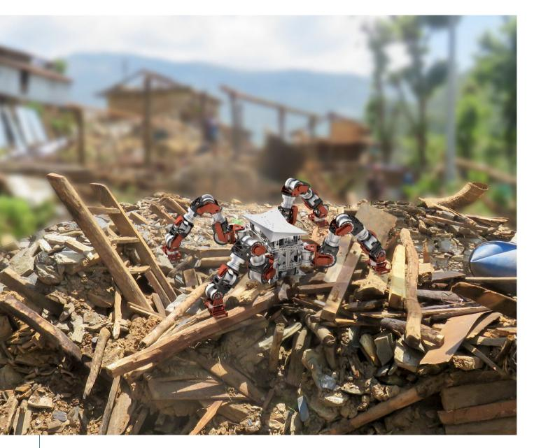
Waseda University's Humanoid Robotics Institute (HRI) has relied on SOLIDWORKS® Research design and engineering software since 2001 to accelerate the pace of robot development. During that time, HRI has introduced 20 humanoid robots, including the WAREC-1 disaster robot (shown here), which features 28 degrees of freedom.
