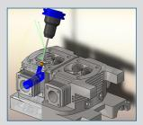
transition from design to toolpath programming, simulation and generating shop floor setup sheets while working inside of both parts and assemblies.
