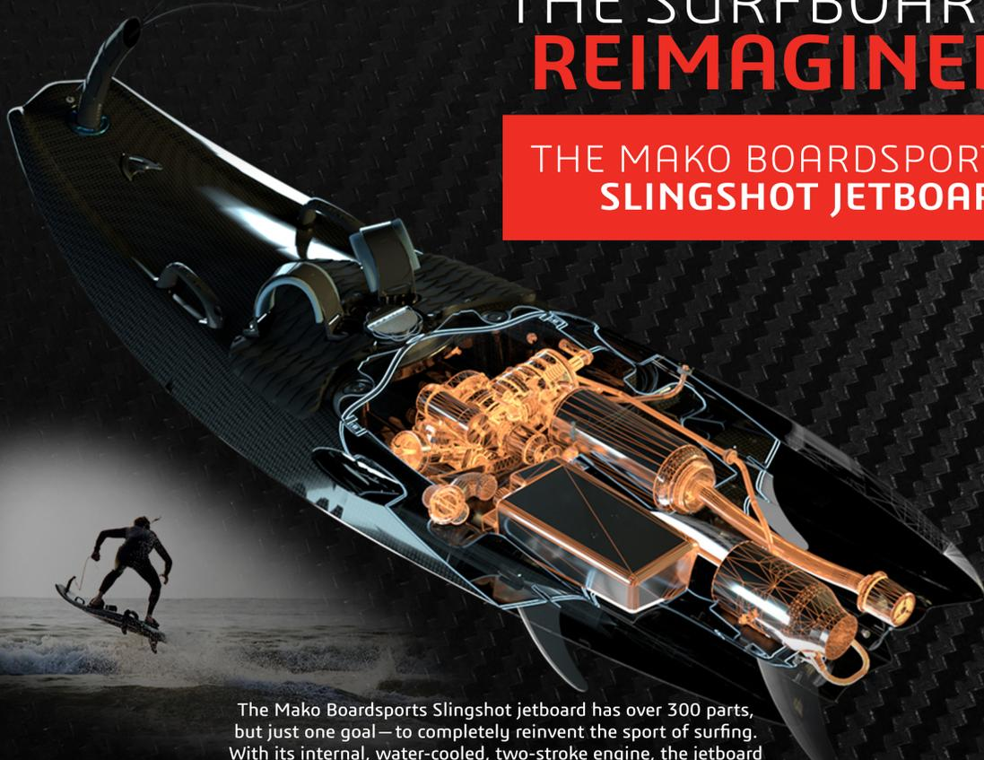
The Mako Boardsports Slingshot jetboard has over 300 parts, but just one goal—to completely reinvent the sport of surfing. With its internal, water-cooled, two-stroke engine, the jetboard can be used on almost any body of water with or without surf. Since aesthetics were a top priority for the design team at Gilo Industries, the engineers started with a predetermined carbon fiber body and worked backwards to ensure all the mechanical elements would work together.
