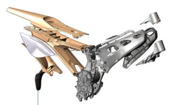
Using SOLIDWORKS Simulation tools, Alta Motors overcame technical challenges while improving motorcycle performance, such as eliminating a third of the design's mass and shaving off an additional 10 percent of its weight, resulting in increased strength and better manufacturability.
