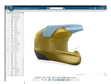
With SOLIDWORKS Industrial Designer software, CAD can easily move back and forth between its ideation/surfacing and production modeling tools, saving the product development consultancy time and money while enabling it to maintain the industrial design aesthetic when designs move on to manufacturing.
