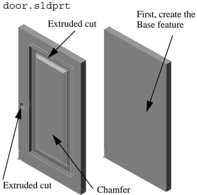
The Chamfer feature is a new feature. The chamfer feature removes material along an edge. It works very similarly to a fillet except the result is a beveled edge rather than a rounded edge.
