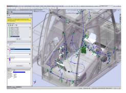
The Landrich harvester cab in SolidWorks/E<sup>3</sup>.WireWorks software.
