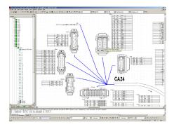
Formboard created in E<sup>3</sup>.series software, infused with flattened 3D layout from SolidWorks software.
