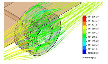
It is now easier to see the turbulence in the airflow between the wheel and car body.
