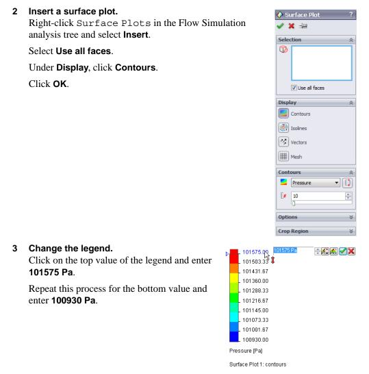
**Note:** The reason we do not use the default values is because if we make a design change to the car and rerun the analysis, the minimum and maximum pressure values will be different. That means red would represent one pressure on one plot and a different pressure on a different plot. Using the same minimum and maximum settings for each analysis allows for meaningful comparisons between different iterations of the design.
