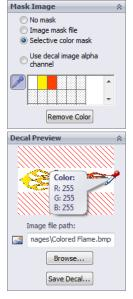
Dragging edges or anywhere inside the frame moves the image, dragging corners resizes, and dragging the center ball rotates.
