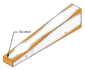
The answer can be found by measuring the blank. The overall length of the blank is 305mm. However, the length of the angled face is about 309mm – about 4mm longer. In order to make a template that is the right size, we need a view that "looks" perpendicular to the angled face. This is called an auxiliary view.
