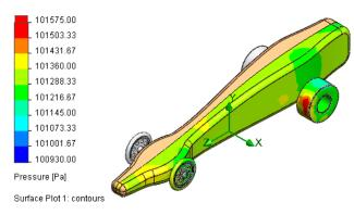
The flow trajectories also provide a clue. There is a significant amount of turbulence surrounding the rear wheels.
