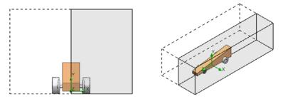
**Note:** Reducing the size of our computational domain and utilizing a symmetry boundary condition will allow for more efficient calculations. We must always be sure, however, that our computational domain is large enough to allow our flow field to fully develop.
