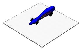
Add a **Tangent** mate between the uppermost face of the **Floor** and the bottom of the wheels. This locates the **Floor** vertically.
