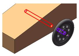
However, this is not the best strategy. A **Coincident** mate requires two planes, either faces or reference planes. If we modify the shape of the car body so that the side is no longer planar, then the **Coincident** mate will fail.
