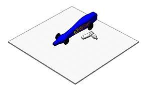
**Tip:** When you get one of the cartridges positioned the way you want it, right-click it and select **Fix** from the shortcut menu. This will lock it in place so it doesn't move when you are positioning the second cartridge.
