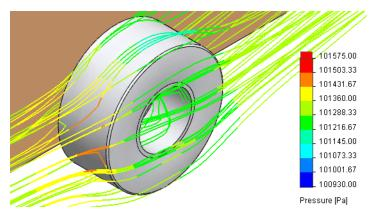
It is hard to see the flow lines between the wheel and the car body because they are obscured by the geometry of the wheel.
