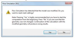
The geometry of the car body has changed. We've rounded the nose and made other changes. The mesh should be reset.
