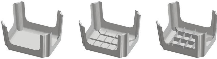
Simulation shows that the shallow rib option actually does meet the structural requirements, such that adding additional material to deepen the ribs contributes nothing but cost to the design.
