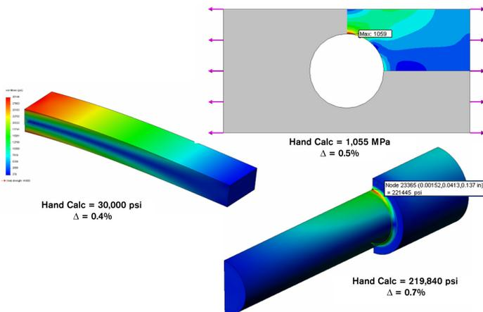
Figure 9: Comparing hand calculations to simulation.
