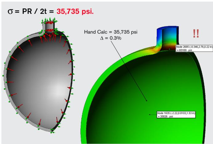
Figure 10: Stress results on a spherical pressure vessel
