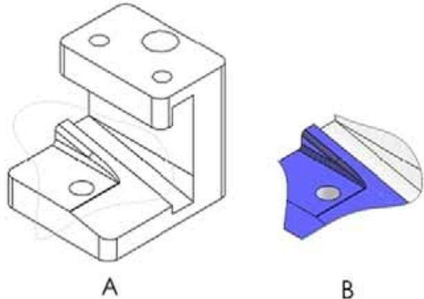
2 To create drawing view 'B' it is necessary to sketch a spline (as shown) on drawing view 'A' and insert which SolidWorks view type?
