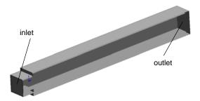
**2** Using the **Wizard**, create the SolidWorks Flow Simulation project for internal water analysis with the **Result resolution** level set to **5** (all other settings are default).
