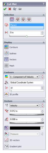
However, the cut plot is not seen through the model. In order to see the plot, you can hide the model by clicking **Flow Simulation**, **Results**, **Display**, **Geometry** (alternatively, you can use the standard SolidWorks **Section View** option) or change the model transparency (as is done in the next step below).
