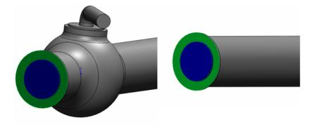
**Note:** In the assembly mode, each newly created lid forms a new part saved in the assembly folder.
