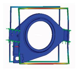
Frequency analysis on a subassembly of a CT scanner
