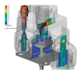
SOLIDWORKS Flow Simulation can simulate the flow of fluids, including non-Newtonian liquids, mixing of fluids, conjugated heat transfer with fluid flow, and external/internal flow. Blood flow provides a good example of a non-Newtonian fluid.
