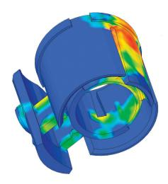
SOLIDWORKS Simulation was used on the injection device's trigger to determine the contact force needed to activate the injection.
