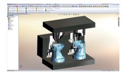
Mold and models in the SolidWorks software/ IMOLD environment
