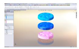
An exploded cavity and core view of a Majesty dispenser lid—gives the designer a preview of how the mold splitting in the SolidWorks software/IMOLD environment.
