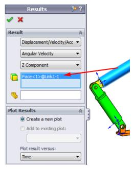
The plot shows the variation of the angular velocity of the center of mass for Link1 as function of time.
