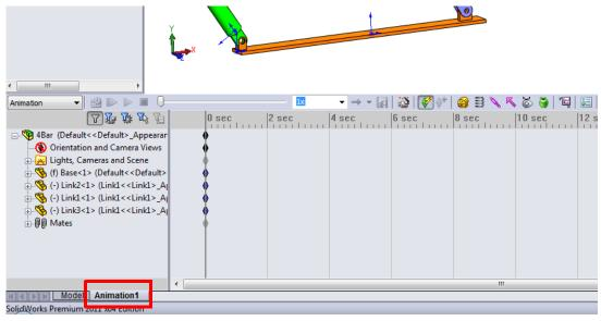
SolidWorks Motion takes full advantage of SolidWorks Animator and thus the look and feel of the SolidWorksMotionManager is very similar to that of the SolidWorks Animator.
