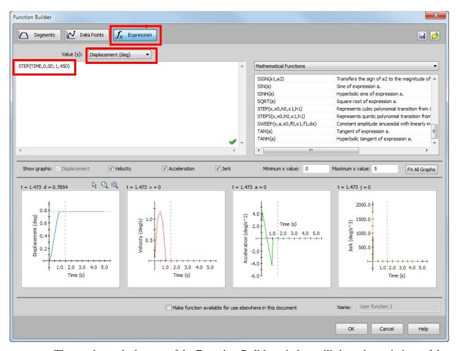
The graphs on the bottom of the **Function Builder** window will show the variations of the displacements, velocities, accelerations and jerk
