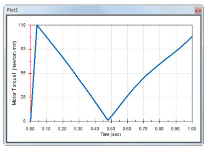
The required torque is about 110 N-mm
