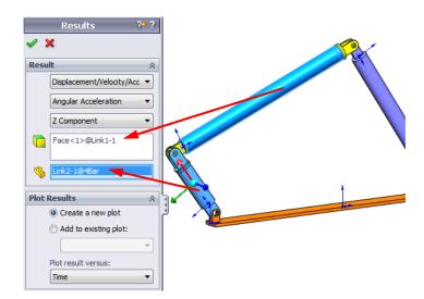
**Note:** The triad on the Link2 component indicates the output local coordinate system. Contrary to the global coordinate system which is fixed, local coordinate systems may rotate. In our case, the selected local coordinate system will rotate because Link2 component rotates as the mechanism moves.
