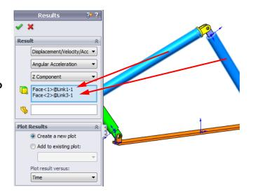
The plot shows the acceleration magnitude of Link1 (its center of mass) with respect to Link3 (part's coordinate system). The maximum relative acceleration is 139 deg/sec^2 in the negative rotational Z direction.
