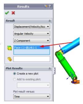
The plot shows the variation of the angular velocity of the center of mass for Link1 as function of time.
