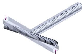
$$\text{Torsional Rigidity} = \frac{\text{Torque Load}}{\text{Angular Deflection}}$$
