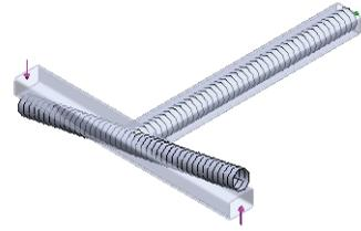
$$\text{Torsional Rigidity} = \frac{\text{Torque Load}}{\text{Angular Deflection}}$$
