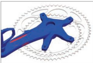
Estimate component life based on calculated loads with fatigue simulation.
