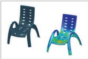
Validate the performance of composite materials, including stiffness and ply failure results.
