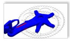
Estimate component life based on calculated or SolidWorks Motion loads.
