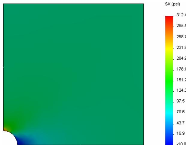
The analytical value for the maximum normal stress is  $\sigma_{\max} = 302.452$  psi.
