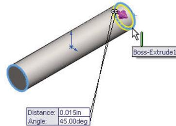
**5 Set the Chamfer distance and angle.**
