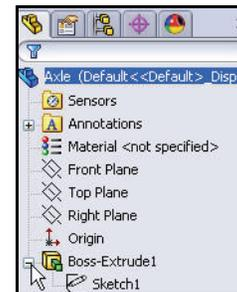
**Note:** With SolidWorks software, it is not necessary to fully dimension or define sketches before you use them to create features. However, you should always fully defined sketches before you consider the part complete for manufacturing.
