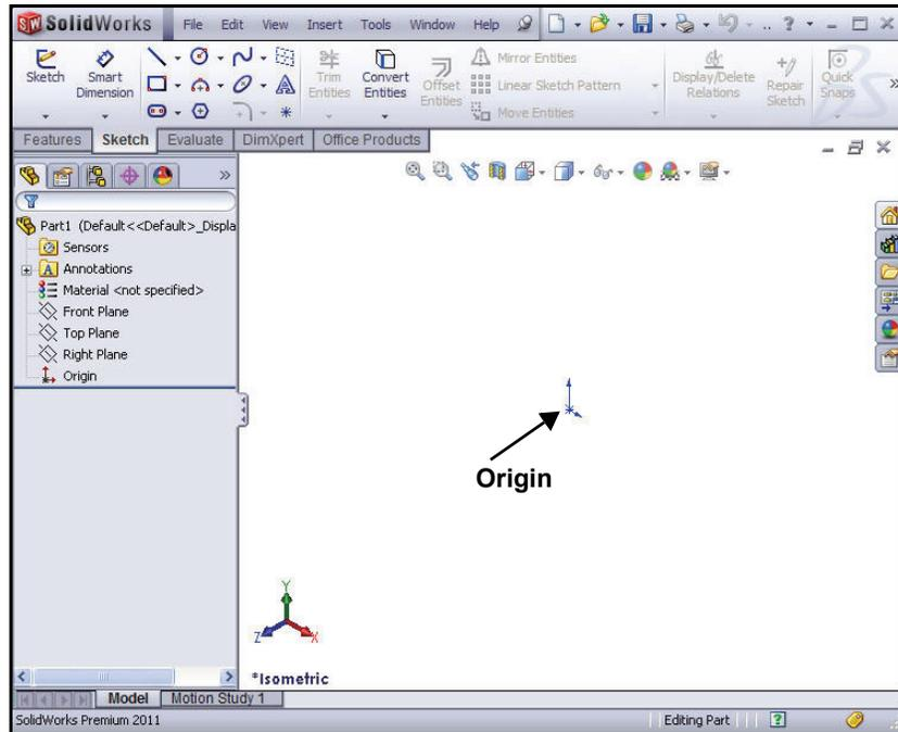
The Reference Triad, (lower left corner) displays the orientation of the model coordinate axes; (red-X, green-Y, and blue-Z) at all times. It can help show how the view orientation has been changed relative to the Front Plane.
