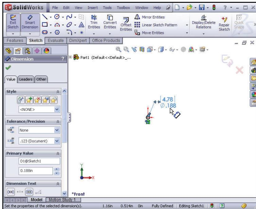
**Note:** The circular sketch is centered at the Origin. The dimension indicates the diameter of the circle is **.188[4.78]**. If your sketch is not correct, select the Undo
