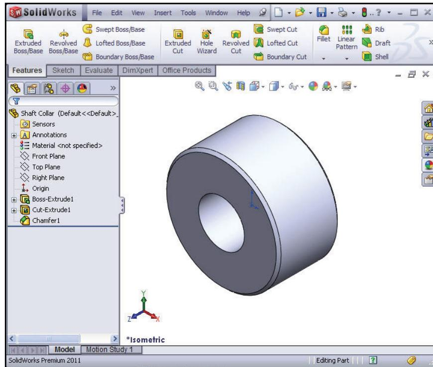
Applying Material to the Shaft Collar
