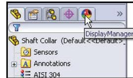
The Shaft Collar DisplayManager is displayed. The DisplayManager tab provides an outline view of the Appearances, Decals and Scene, lights, and cameras effects associated with the active SolidWorks part or assembly.
