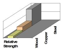
**Note:** Metals are manufactured products and due to the way they are created, they have equal strength in each direction. Materials like this are called *isotropic* materials.
