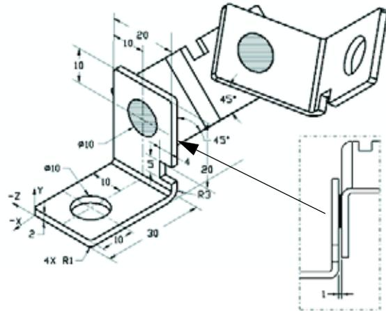
**Brackets:** 2mm thickness, and equal size (holes through-all). Material: 6061 Alloy, Density =  $0.0027\text{g/mm}^3$ . The top edge of the notch is located 20 mm from the top edge of the MachinedBracket.
