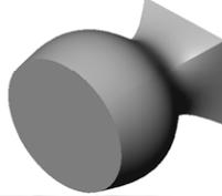
**A Second Loft Feature Creates the Bit of the Chisel:**
