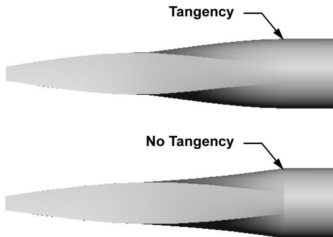
In the **Start/End Constraints** box of the PropertyManager, there are some tangency options. **End constraint** applies to the last profile, which in this case, is the face on the end of the shaft.
