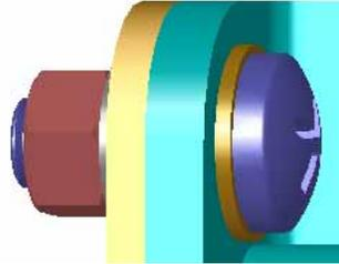
To add these parts to an assembly, select the type of part you want to insert, then drag the Toolbox part into your assembly. As you drag Toolbox parts, they snap to the appropriate surfaces — automatically establishing a mate relationship. In other words, a screw recognizes that it belongs in a hole and snaps to it by default.
