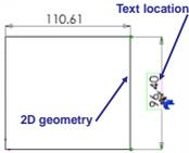
The diagram shows a 2D sketch of a rectangle with a horizontal dimension of 110.61 and a vertical dimension of 26.40. Arrows point to the '2D geometry' and 'Text location' for each dimension. The background shows a faint image of a mechanical part.
