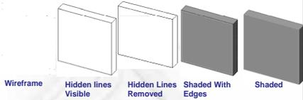
Wireframe   Hidden lines Visible   Hidden Lines Removed   Shaded With Edges   Shaded
