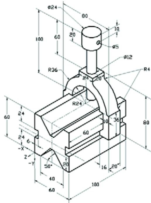
What is the center of mass of the assembly with respect to the illustrated coordinate system?
