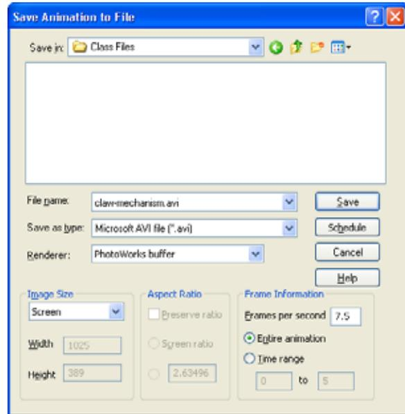
**Note:** The file types \*.bmp and \*.avi increase in file size as more appearances and advanced rendering effects are applied. The larger the image size the more time is required to create the image and animation files.
