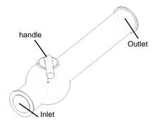
The standard engineering definition of a hydraulic resistance of an obstacle in a pipe is the difference between the total pressures (i.e. where a stream is not disturbed by the obstacle) upstream and downstream of the obstacle (the valve in our case) divided by the incoming dynamic head, from which the hydraulic resistance due to the friction over the pipe section is subtracted.
