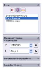
By specifying this condition we define that the water has a static pressure of **1 atm** at the ball valve pipe exit.
