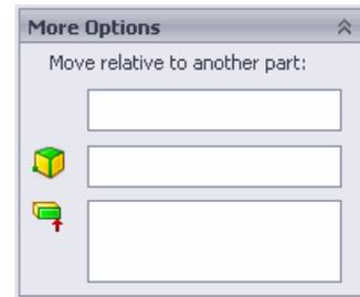
Because the default location of the motor, determined by the cylindrical face specified in under **Component/Direction** is correct, **Motor location** field under **More options** will be left blank as well.
