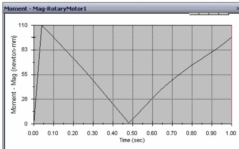
The required torque is about 110 N-mm
