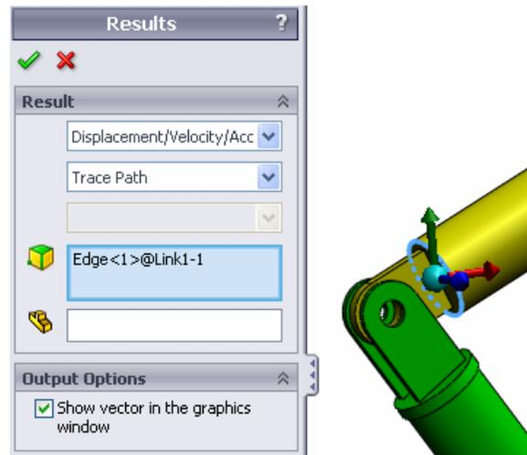
Note that the resulting trace path is by default shown with respect to the fixed ground. To show the trace path with respect to another moving component, one would have to select this reference component as a second item in the same selection field.
