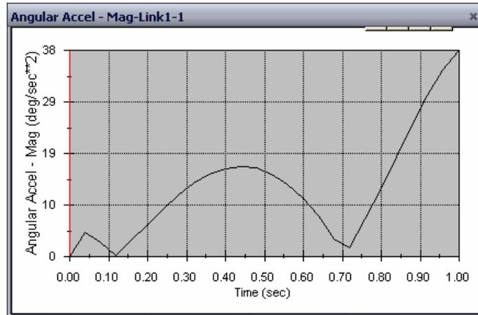
The results indicate the maximum angular velocity and angular acceleration of 6 deg/sec and 38 deg/sec<sup>2</sup>, respectively.
