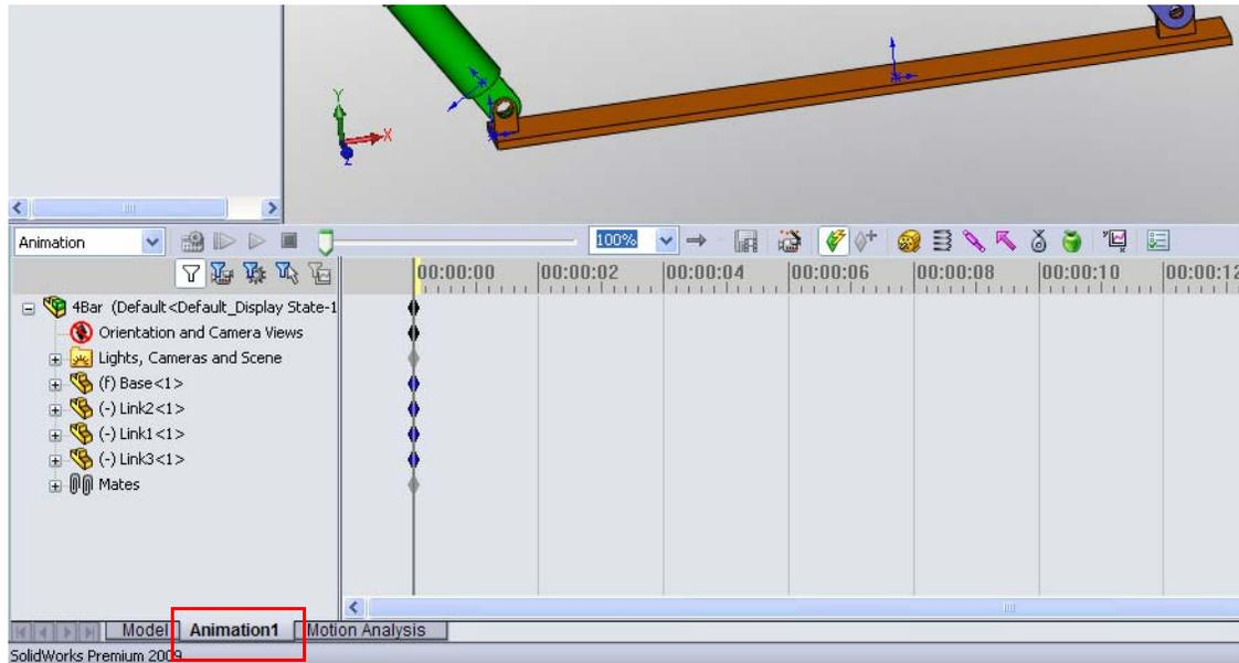
SolidWorks Motion takes full advantage of SolidWorks Animator and thus the look and feel of the SolidWorksMotionManager is very similar to that of the SolidWorks Animator.
