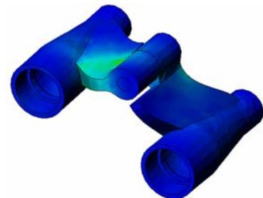
Optimization studies are applied to improve (optimize) your initial design based on a set of selected criteria such as maximum stress, weight, optimum frequency, etc. Typical questions that will be answered using this study type are:
