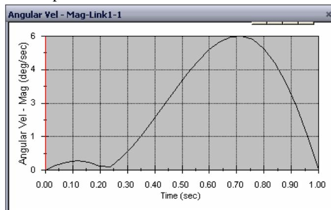
The above plot shows the variation of the angular velocity of the center of mass for Link1 as function of time.
