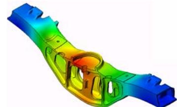
Buckling studies analyze performance of the thin parts loaded in compression. Typical questions that will be answered using this study type are:
